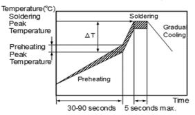
[ Allowable Flow Soldering Temperature and Time ]
