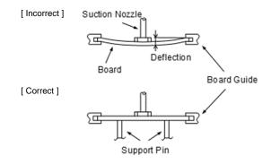
2. Dirt particles and dust accumulated in the suction nozzle and suction mechanism prevent the nozzle from moving smoothly. This creates excessive force on the capacitor during mounting, causing cracked chips. Also, the locating claw, when worn out, imposes uneven forces on the chip when positioning, causing cracked chips. The suction nozzle and the locating claw must be maintained, checked and replaced periodically.
