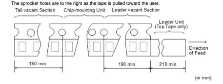
5. Accumulate tolerance of sprocket holes pitch = +/-0.3mm/10 pitch
