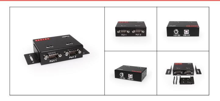
2-port USB to Serial 9 Pin RS-232 Industrial adapter with Surface or Din Rail mounting Configuration. Surface Visible Power and Activity LED's for easy diagnostic review. Utilizes FT2232H FTDI Chip set Automatically configures the additional COM ports Plug and Play allows easy installation Perfect for connecting serial modems, bar code scanners, CNC routers, and others Rugged metal industrial design
