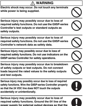
required safety functions. Ground the 0V line of the power supply for external output devices so that the devices do NOT turn ON when the safety output line or the test output line is grounded.
