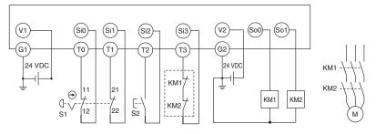
Emergency stop switch Reset switch KM1, KM2: Magnetic contactors Motor
