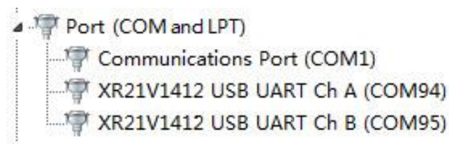
Figure 5: UART Ports Displayed on PC
