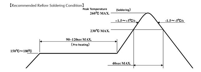
Note 1 Recommended temperature profile for the reflow soldering is listed as the temperature of the resin surface. This should be the maximum temperature for soldering. Lowering the heating temperature and decreasing heating time is very effective in achieving higher reliability.
