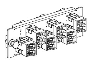
6 POSITION DUPLEX E2000 FIBER ADAPTER PANEL CUSTOMER DRAWING
