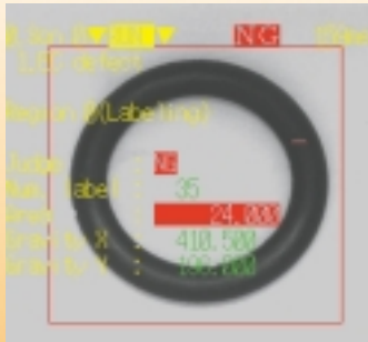
Correctly detects distortion or deformation in rubber packing, etc.
