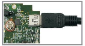
Connect the USB mini-B cable to J1
