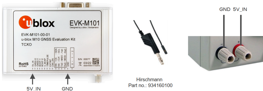
Figure 3: EVK-M101/C 5.0 V DC power supply example
