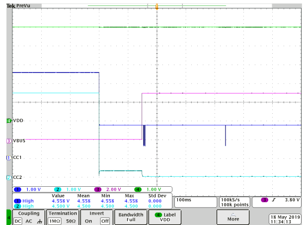
Figure 53. VCONN when Cable Marker Cable is Attached (FUSB3307 w/3A Support)
