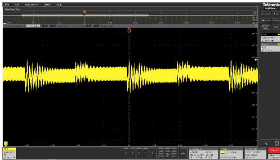
Figure 24. Transient Load on 5 V BUS
