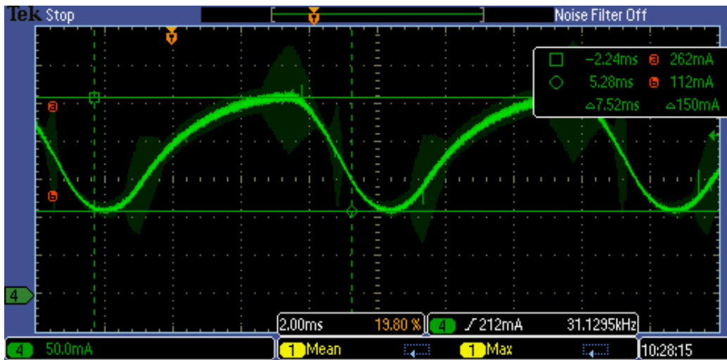
Figure 14. Output Ripple 75% Pk - Pk
