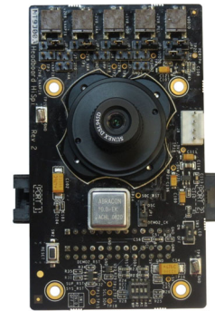
Figure 1. MT9J003 Evaluation Board
