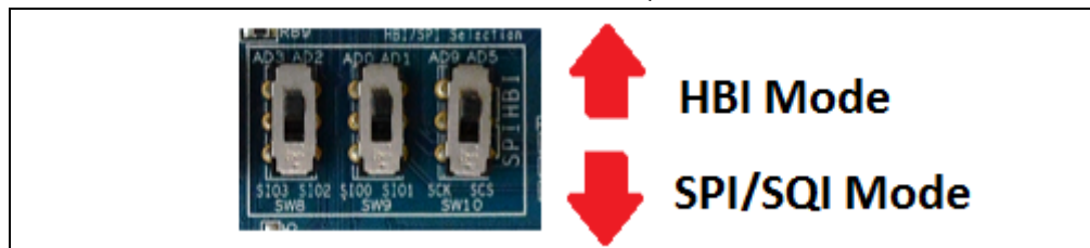
FIGURE 3-3: SW8-SW10 HBI AND SPI/SQI MODE SELECTION
