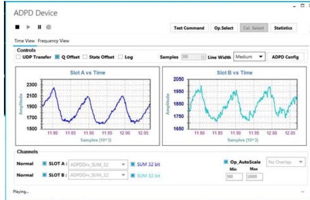
Figure 8. Example of a PPG Signal
