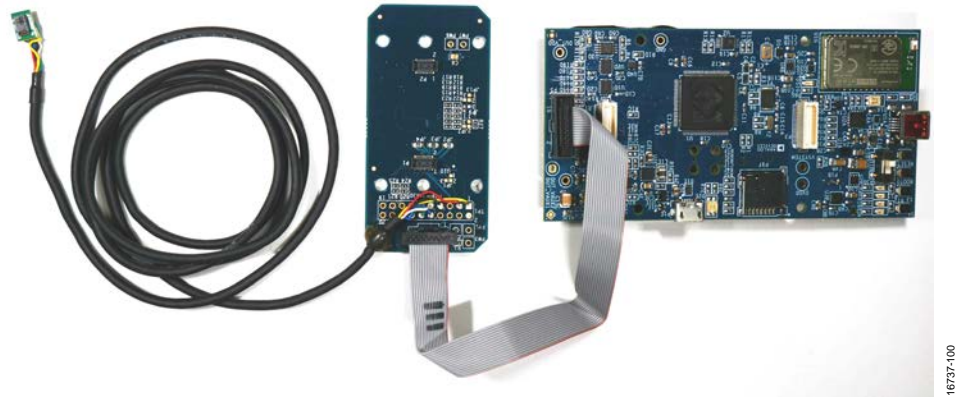
Figure 15. EVAL-ADPD144RIZ-SF Connected to the EVAL-ADPDUCZ Microcontroller Board
