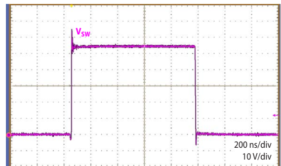
Figure 7: Measured switch-node voltage at V_{IN} = 56V, V_{OUT} = 20V, I_{OUT} = 12.5A
