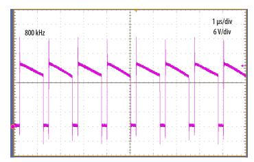
Figure 9: Switch-node waveform at 48 V input to 19 V, 12.5 A output
