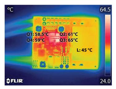
Figure 11: Thermal image of the EPC9148 at 48 V input to 19 V, 12.5 A output with 800 LFM forced air
