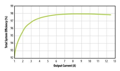
Figure 10: Total system efficiency as a function of the output current at 48 V input to 19 V output
