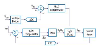
Figure 6. Block diagram of the average current mode controller (ACMC) with flying capacitor voltage adjust duty cycle control input.
