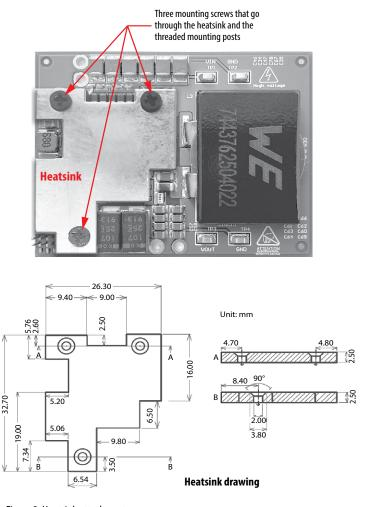
Figure 8: Heatsink attachment
