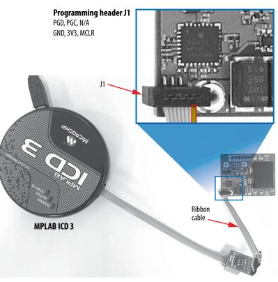
Figure 12: Programming connection
