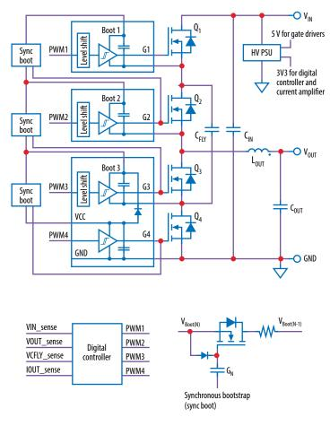
Figure 1: Block diagram of the EPC9148 demonstration board
