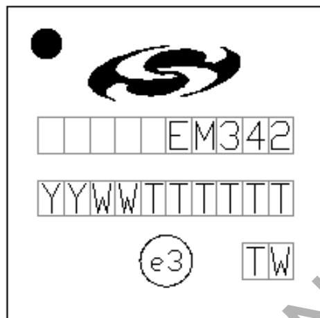
Figure 19.1. Part Marking for EM342
