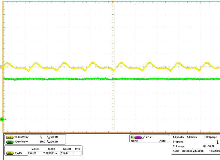
Figure 7: Ripple, V_{IN} = 12V , V_{OUT} = 0.9V , I_{LOAD} = 30A , f_{SW} = 800\text{ kHz}
