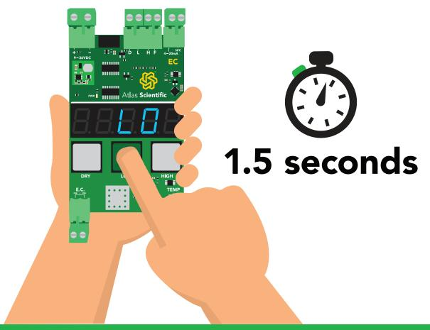
The conductivity readings will not change after low point calibration. The readings will change only when both high and low point calibration has been completed.
