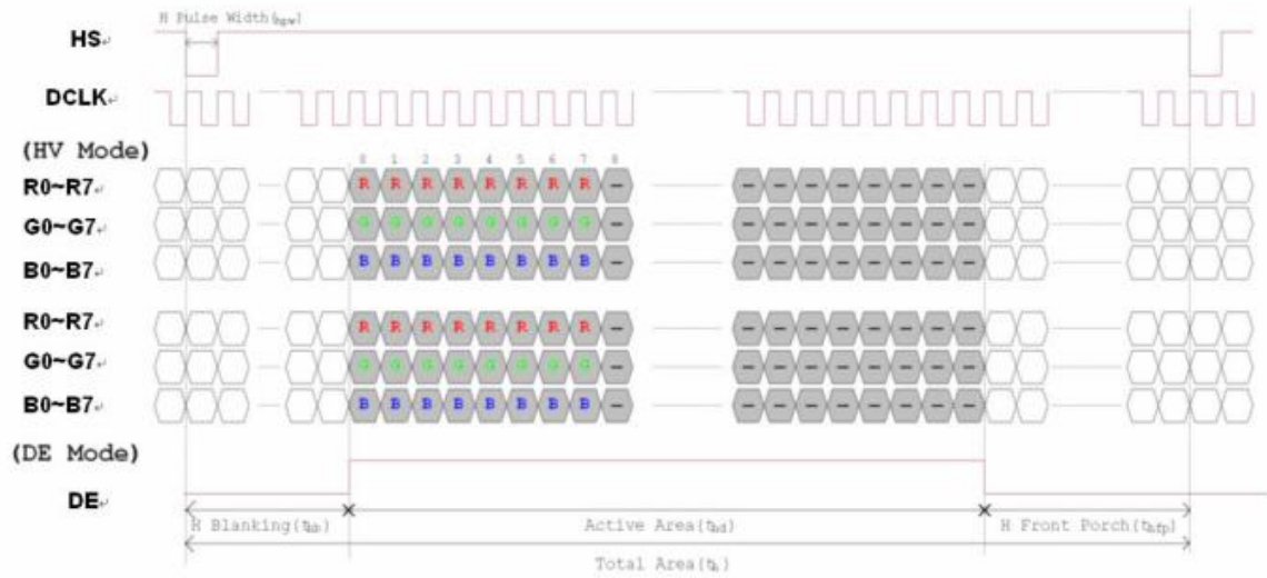
Figure 3. 1 Horizontal input timing diagram.
