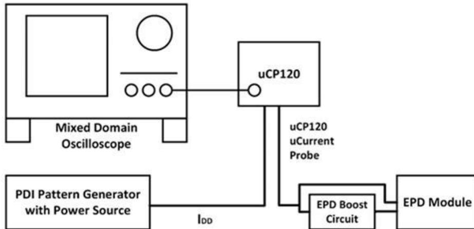
\*Set oscilloscope filter > 200MHz and record length to 10M points.
