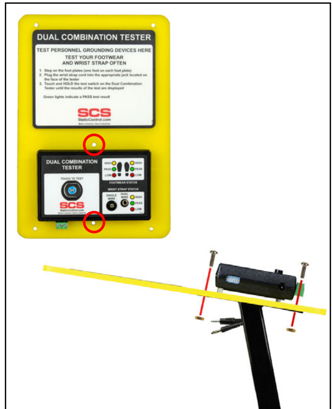
Figure 6. Securing the Dual Combination Tester to the pedestal
