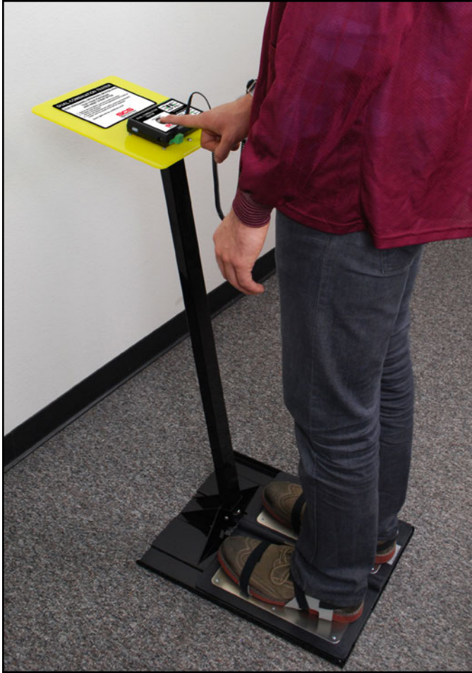
Figure 12. Using the Dual Combination Tester with 770755 Stand
