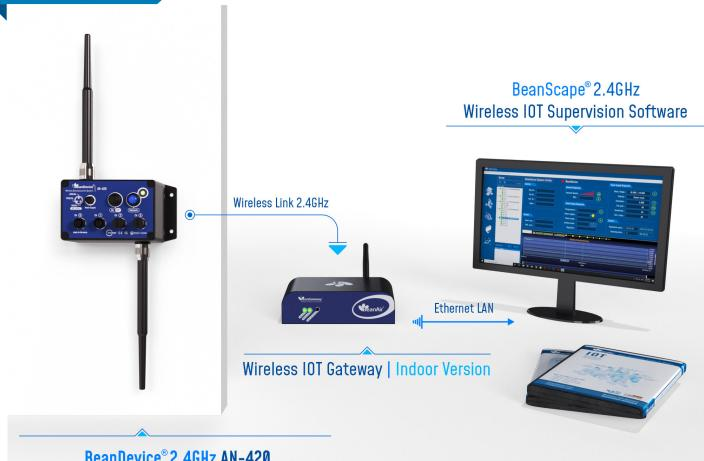
BeanDevice<sup>®</sup> 2.4GHz AN-420 Wireless IOT Data Acquisition (DAQ) Instrument 4-20mA (current loop) inputs
