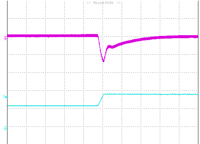
Figure 9: Output voltage response to step-change in load current (50%-75% of I_o , max; di/dt = 0.1A/\mu s , V_{in}=48V ). Load cap: 220 \mu F , electrolytic capacitor ; 10 \mu F , tantalum capacitor and 1 \mu F ceramic capacitor. Top Trace: V_{out} (200mV/div, 200us/div); Bottom Trace: I_o (10A/div, 200us/div). Scope measurement should be made using a BNC cable (length shorter than 20 inches). Position the load between 51 mm to 76 mm (2 inches to 3 inches) from the module..
