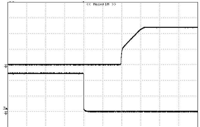
Figure 20: Turn on delay time at remote on 12Vin, 1.2V/12A out. (Top: VOUT, 0.5V/div; Bottom: ON/OFF, 2V/div; 2mS/div)
