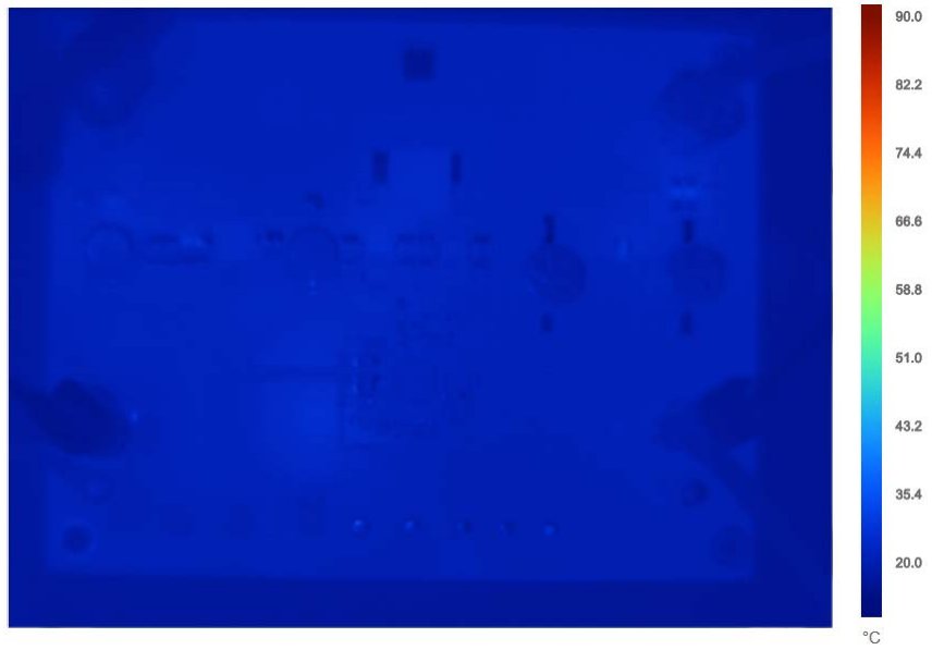
Figure 15. DC2814A-A Thermal Performance at 12V IN (Pass-Thru), 12V OUT , 3A Load Current
