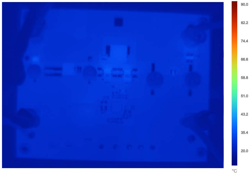
Figure 9. DC2814A-A Thermal Performance at 6V IN (Boost), 8V OUT , 3A Load Current
