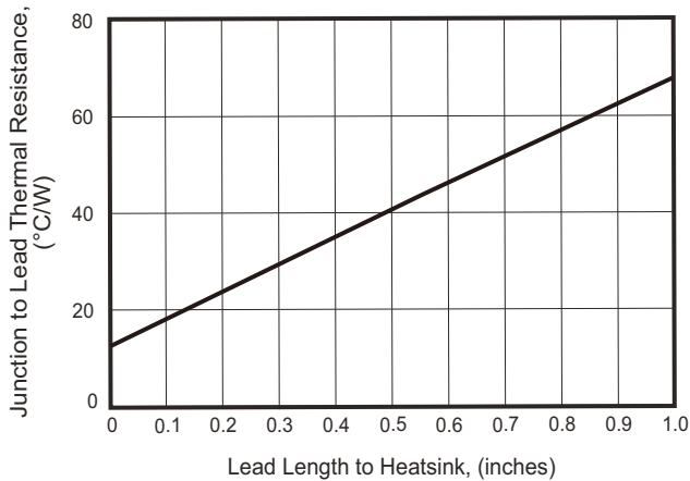
Fig.3 - Typical Thermal Resistance v.s. Lead Length
