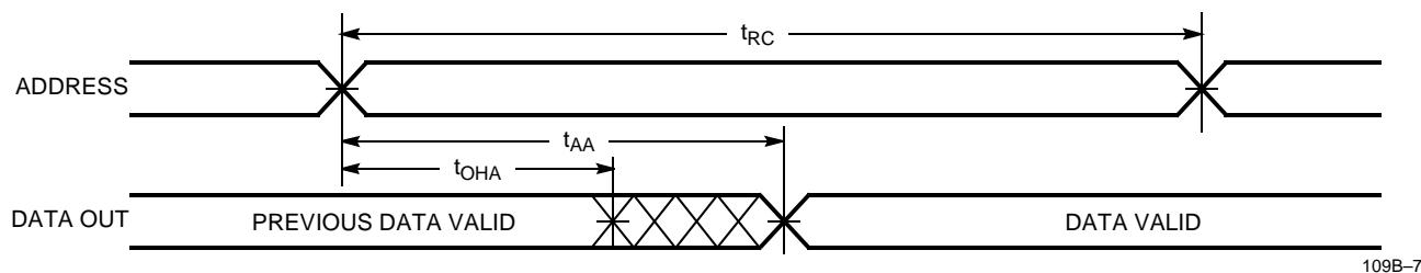
Read Cycle No. 2 ( $\overline{OE}$  Controlled)<sup>[11, 12]</sup>
