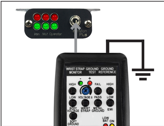
Figure 25. Connecting the Verification Tester to the Ground Man Plus Workstation Monitor's operator jack
