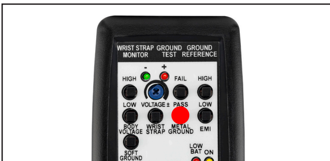
Figure 21. Pressing the METAL GROUND PASS test switch
