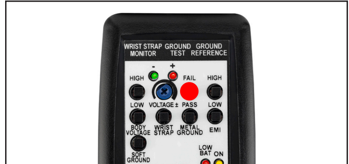
Figure 22. Pressing the METAL GROUND FAIL test switch
