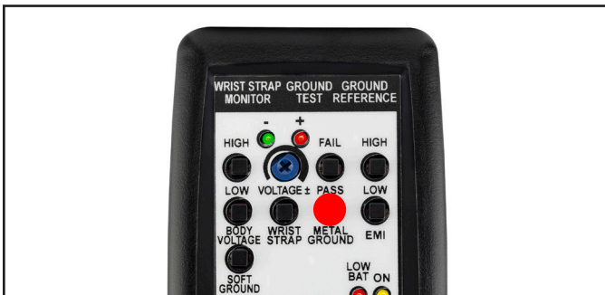
Figure 30. Pressing the METAL GROUND PASS test switch
