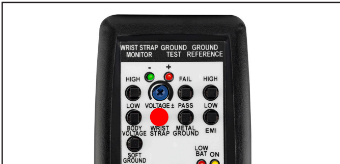
Figure 4. Pressing the WRIST STRAP test switch
