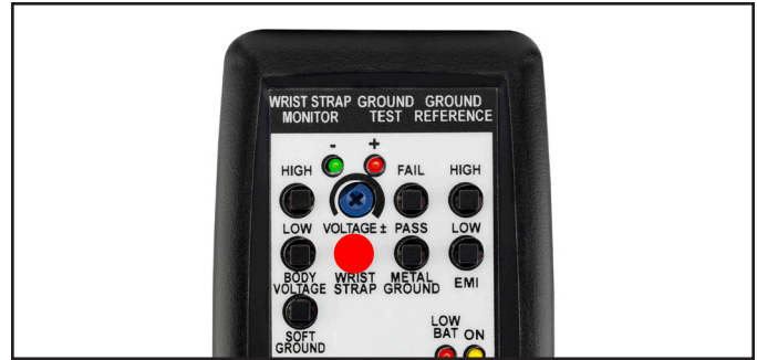
Figure 26. Pressing the WRIST STRAP test switch
