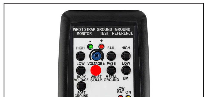
Figure 10. Pressing the WRIST STRAP test switch
