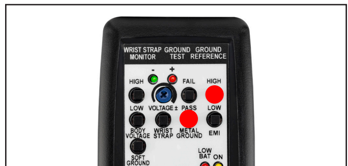
Figure 33. Pressing the METAL GROUND PASS and EMI HIGH test switches simultaneously
