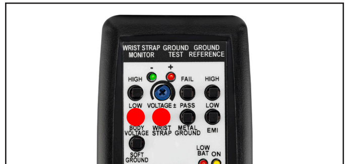
Figure 27. Pressing the WRIST STRAP and LOW BODY VOLTAGE test switches simultaneously
