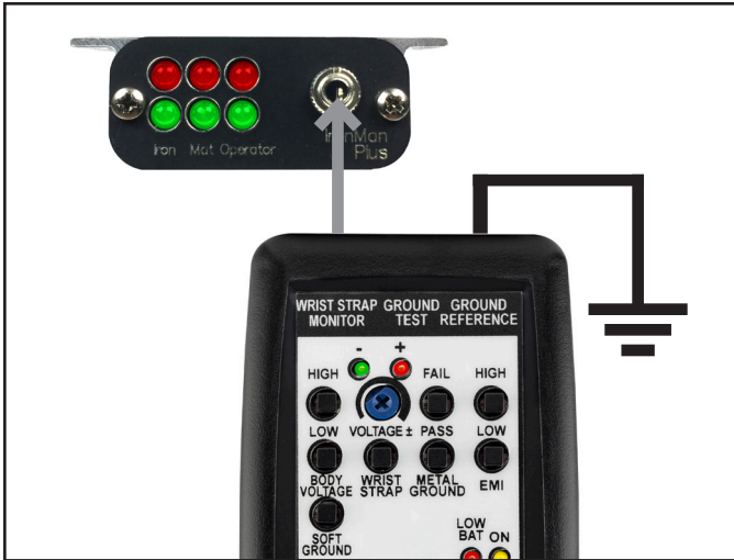
Figure 3. Connecting the Verification Tester to the Iron Man® Plus Workstation Monitor's operator jack
