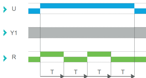
Function Di - Flasher (Symmetrical) – ON Start
