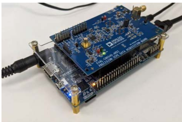
Figure 18. EVAL-CN0540-ARDZ Mounted on Terasic DE10-Nano Carrier Board
