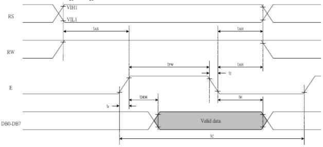
Write cycle (Ta=25°C, VDD=2.7V)
