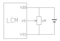
$V_{\text{DD-}}V_0\text{: LCD Driving voltage}$
