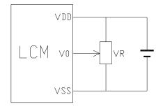
V<sub>DD~</sub>V<sub>0</sub>: LCD Driving voltage
