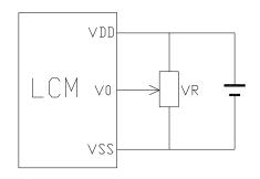
VDD~V0: LCD Driving voltage
