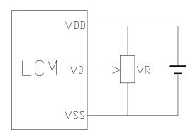
VDD~V0: LCD Driving voltage
