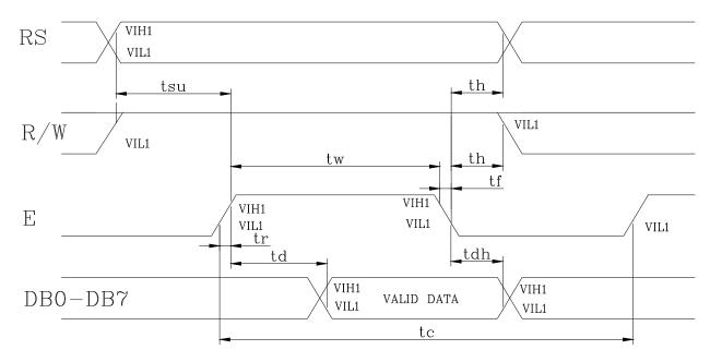
Write cycle (Ta=25°C, V<sub>DD</sub>=5.0V)
