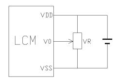
V<sub>DD~</sub>V<sub>0</sub>: LCD Driving voltage
