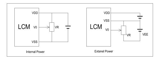
$V_{DD-}V_0$ : LCD Driving voltage VR: 10k~20k
