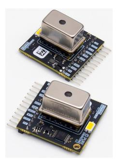
All power and signal pins on the C12880MA Breakout Board have been conveniently broken out so it is easy to connect via jumper or breadboard to any system of your choice. This breakout board features a super bright white LED for illuminating a target to measure fluorescence responses.
