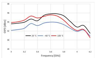
Figure 25. OIP3 @ VDD = 5V : ATT = 15dB, Output = +3dBm/tone, 100MHz interval
