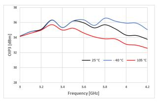
Figure 26. OIP3 @ VDD = 3.3V : ATT = 15dB, Output = +3dBm/tone, 100MHz interval
