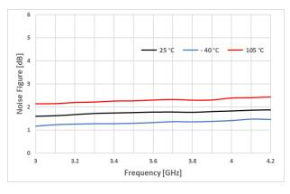
Figure 38. Noise Figure : VDD = 5V, ATT = 15dB
