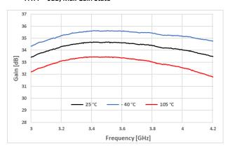
Figure 8. Gain Flatness @ VDD = 3.3V : ATT = 0dB, Max Gain State
