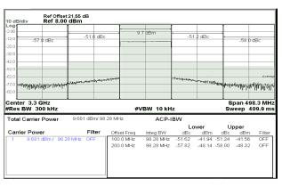
Figure 32. ACP @ 3.3GHz, VDD = 3.3V : ATT = 0dB, 5GNR 100MBW, PAR = 9.6dB
