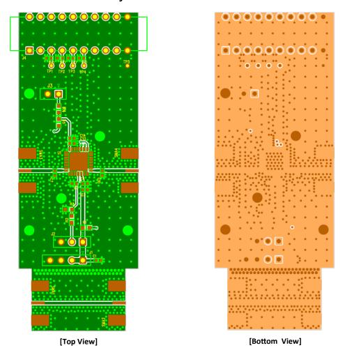
Figure 43. Evaluation Board PCB Layer Information
