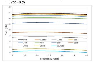
Figure 12. Gain vs Attenuation Settings
