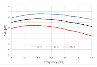
Figure 10. Gain Flatness @ VDD = 3.3V : ATT=31.75dB, Min Gain State
