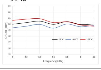
Figure 28. OP1dB @ VDD = 3.3V : ATT = 0dB
