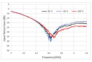
Figure 14. Input Return Loss : VDD = 5.0V, Min Gain State
