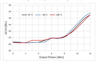
Figure 31. ACP @ 3.3GHz, VDD = 5.0V : ATT = 0dB, 5GNR 100MBW, PAR = 9.6dB
