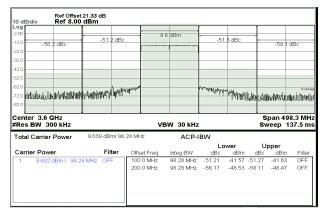
Figure 34. ACP @ 3.6GHz, VDD = 3.3V : ATT = 0dB, 5GNR 100MBW, PAR = 9.6dB
