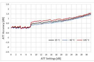
Figure 21. Attenuation Error
