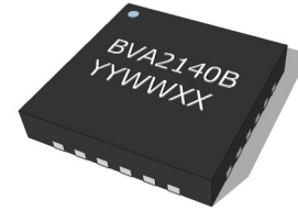
24-lead 4mm x 4mm x 0.9mm QFN
