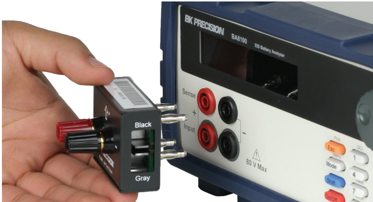
TLC81 plugged-in to the front panel
