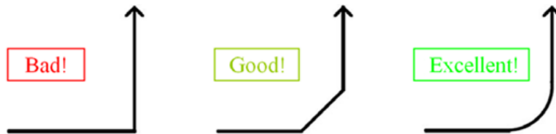
Figure 5-13: Examples of Turns in Trace Routing
