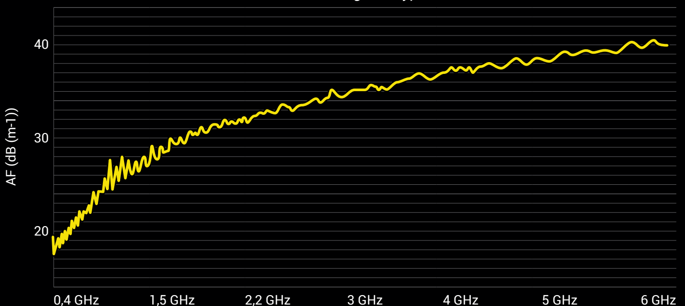
Antenna Factor Diagram HyperLOG® 4060
