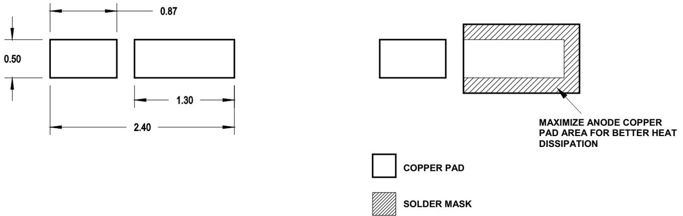
NOTE: All dimensions are in millimeters (mm).
