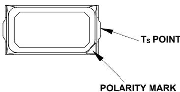
$T_S$  can be easily measured by mounting a thermocouple on the soldering joint as shown in preceding figure, while  $R_{\theta J-S}$  is provided in the data sheet. Verify the  $T_S$  of the LED in the final product to ensure that the LEDs are operating within all maximum ratings stated in the data sheet.
