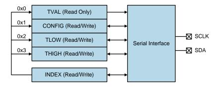
For additional configuration settings the Config register (0x1) has to be addressed. Please refer the data sheet for details.
