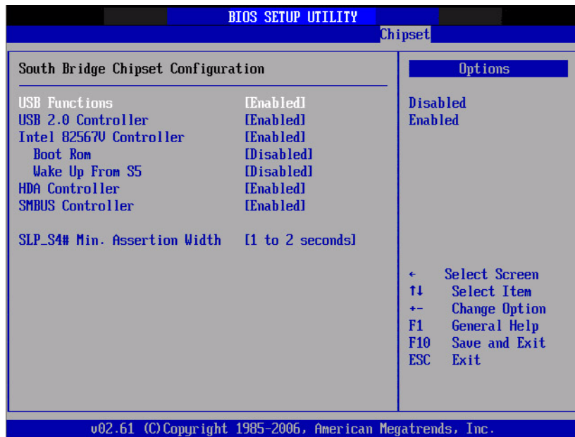
Figure 3.26 South Bridge Configuration
