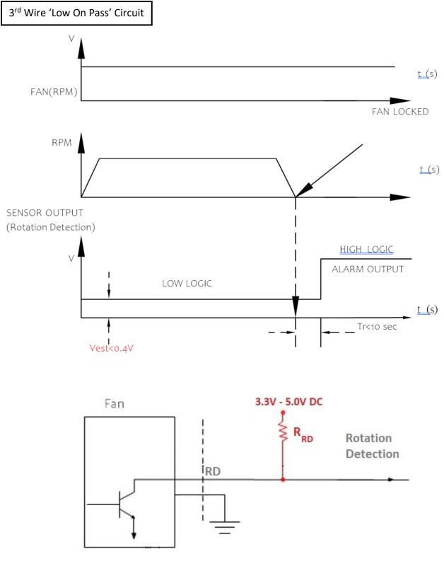
NB: Suggested pull-up resistor value of 1K to  $10 \text{K}\Omega$
