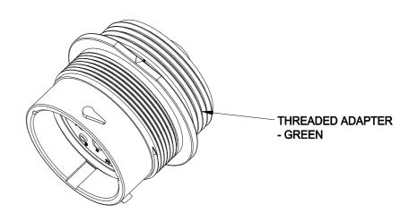
RECEPT,24-14 POS, PIN CONT,NOMAL WTA. SEAL, AHDP
