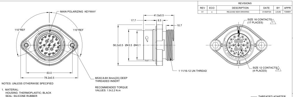
2. MODIFICATIONS: WIDE THREAD ADAPTOR (WTA); REDUCED DIA. WIRE SEAL SEALED PANEL MOUNT
